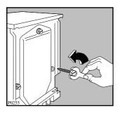
Remove the polystyrene base and take off the bottom panel by unscrewing the central screw. Carefully slide out the right polythene bag.
